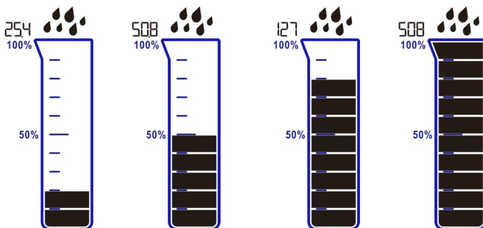
The cylinder chart shows the amount of precipitation in real time, irrespective of the active display mode. The cylinder is divided into 10 segments. Every segment symbolises 10% of the current cylinder capacity (value A11, mm or in, depending on previously selected settings). As of the moment of exceeding 100%, the total cylinder capacity is increased and the percentage values (segments) will be updated automatically.
